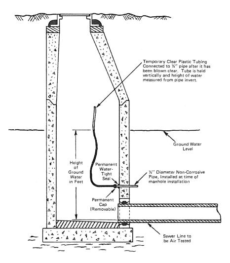
AIR TEST DATA SHEET PIPE TESTING FORM NOTE: Pressurize pipe to 4.5 P.S.I.F. and let stabilize for 5 minutes. Pressure should then be backed off to 4.0 P.S.I.G. and test time started.
