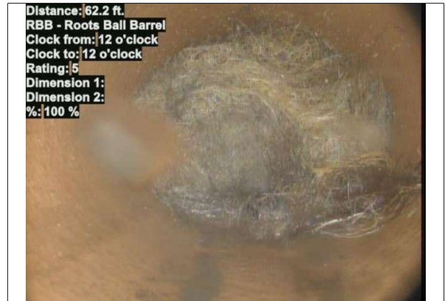
At: 62.2 ft. RBB - Roots Ball Barrel 12/12 Joint: No 100 %
